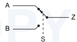
Figure 1-7 Switch model for multiplexer function.
