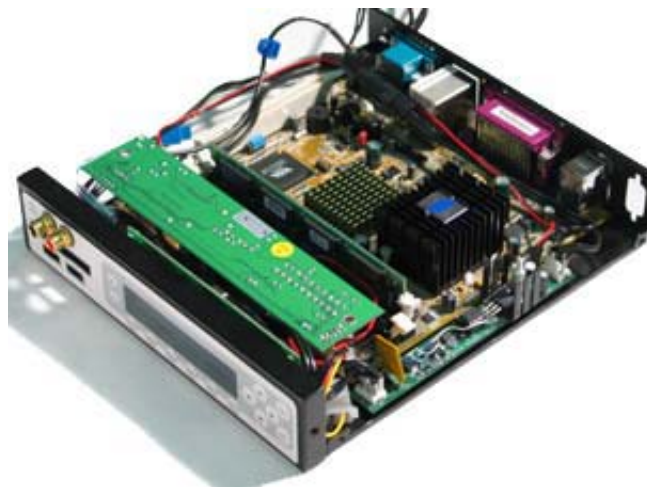
Fig 2.3 ITPS mounted in the mini-box M-100
