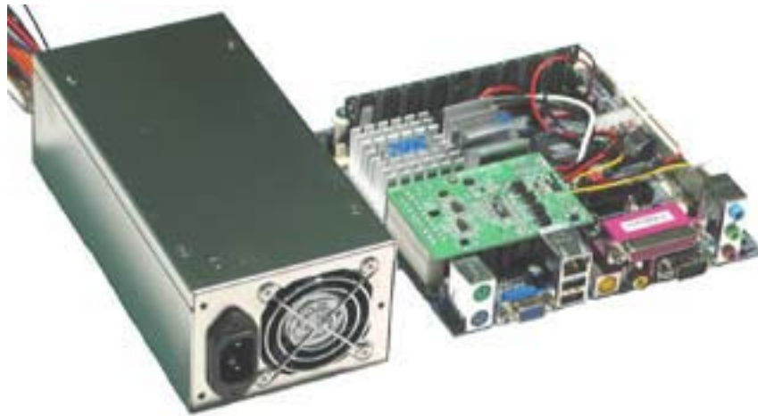
Fig 1.3 - Typical ATX power supply next to an EPIA-M with a micro PSU.
