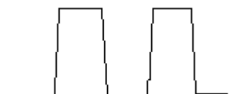
图 6 Schmitt 触发器的输出波形 Fig.6 Output waveform of schmitt trigger
