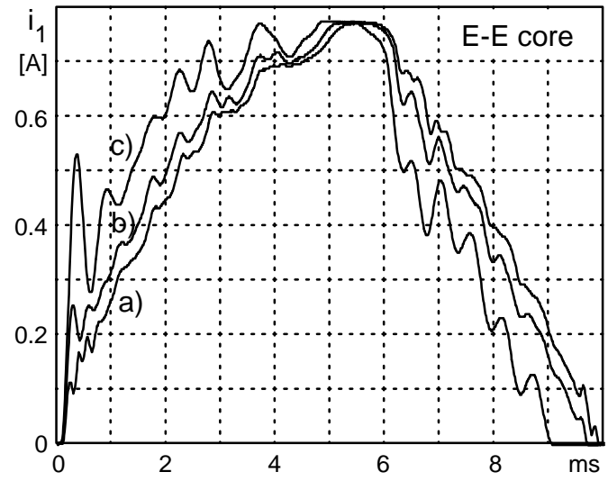
Fig.10 - Input current waveforms for different C_1 values (nominal conditions): a) 220nF, b) 680nF, c) 2uF
