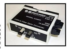
The CAN side is connected to the system through terminal blocks. The fiber is connected though ST connectors. A power supply of 10-30 VDC is required. Model CANFB is housed in a rugged DIN-Rail mountable box, making it easy to install in an industrial cabinet.
