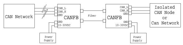
The CAN network must be terminated at both ends according to the CAN specification. Networks not properly terminated may have data errors or miss the data completely. The CANFBs create two new ends to the CAN network. Space is provided on the board for a termination resistor, R8. A 120-ohm resistor is recommended for the termination. If the CANFB is not at the end of the network, it should not be terminated.
