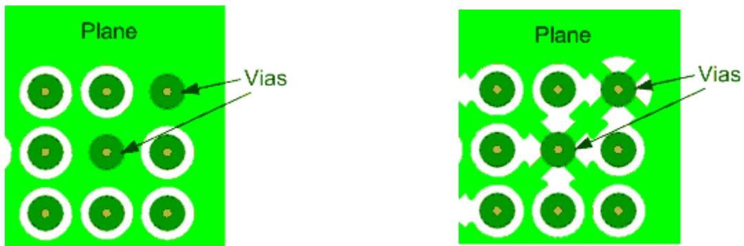
a. Direct via connection to the plane
