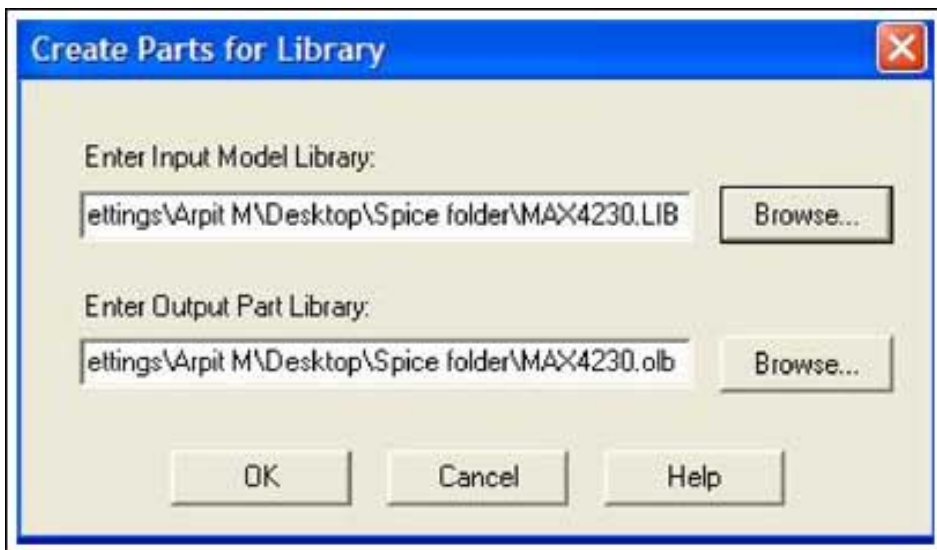
Figure 2. The creation of a Spice model symbol starts at the Create Parts window.
