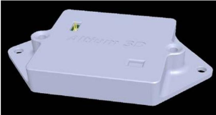
Figure 13. Multivibrator PCB fully assembled into two part housing assembly.
