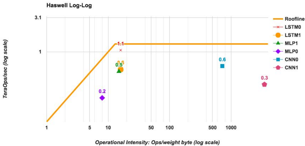
Figure 6. Intel Haswell CPU (die) roofline with its ridge point at 13 operations/byte, which is much further left than in Figure. 5. LSTM0 and MLP1 are faster on Haswell than on the K80, but it is vice versa for the other DNNs.
