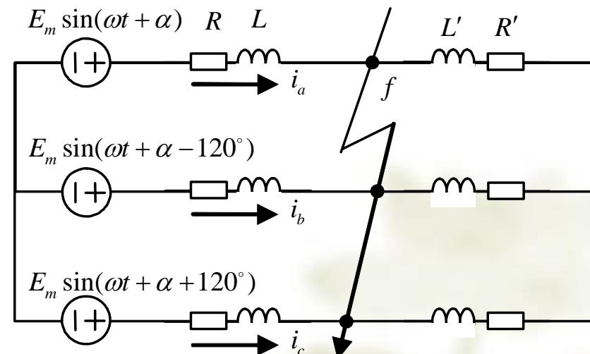
$$I_{pm} = \frac{E_m}{\sqrt{R^2 + (\omega L)^2}}; \quad \varphi = \arctg \left( \frac{\omega L}{R} \right); \quad \lambda = -\frac{R}{L}; \quad T_a = \frac{L}{R}$$
