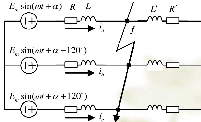
$$I_m = \frac{E_m}{\sqrt{(R + R')^2 + \omega^2(L + L')^2}}; \quad \varphi' = \arctg \frac{\omega(L + L')}{R + R'}$$
