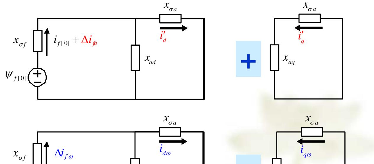
$$\left. \begin{aligned} i_{abc(ap)} \\ i_{abc(2\omega)} \\ \Delta i_{f\omega} \end{aligned} \right\} \Leftrightarrow \left. \begin{aligned} i_{d\omega} \\ i_{q\omega} \\ \Delta i_{f\omega} \end{aligned} \right\}$$
