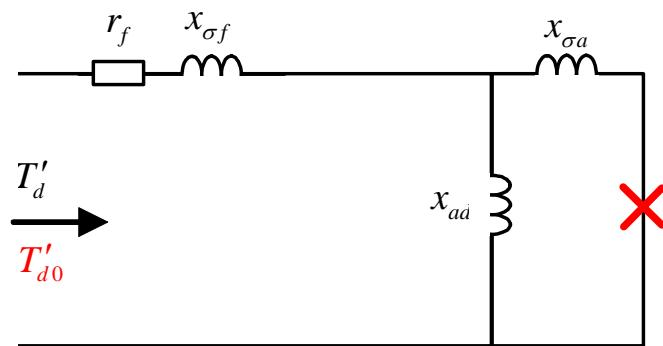
纵轴暂态开路时间常数:  $T_{d0}' = \frac{x_f}{\omega r_f}$
