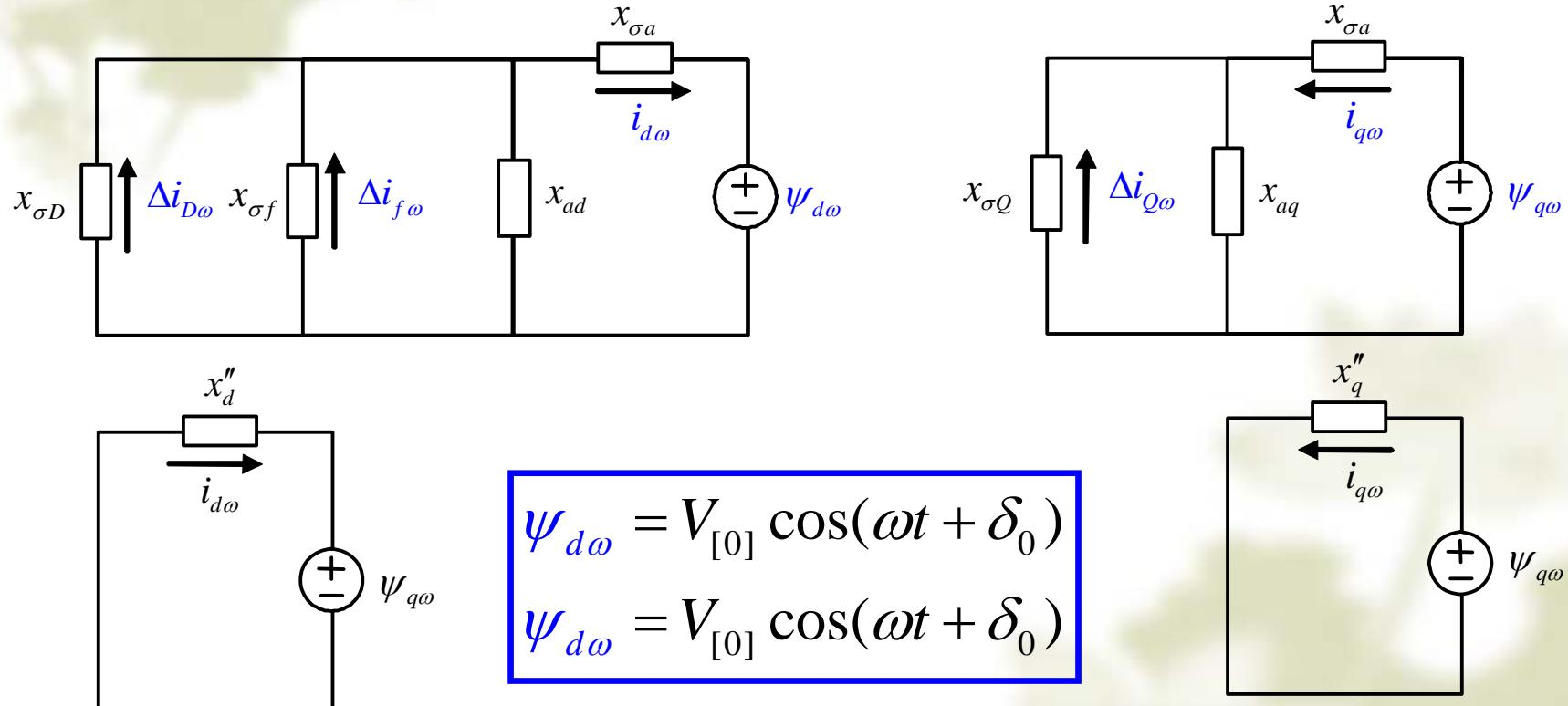
$$i_{d\omega} = -\frac{\psi_{d\omega}}{x_d''} = -\frac{V_{[0]}}{x_d''} \cos(\omega t + \delta_0)$$
