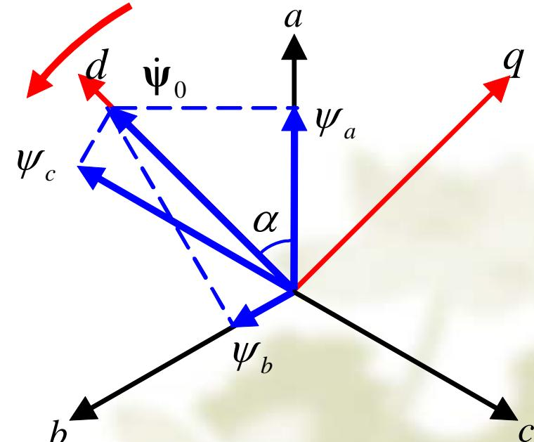
$$\psi_a = \Psi_0 \cos(\omega t + \alpha_0), \quad \psi_b = \Psi_0 \cos(\omega t + \alpha_0 - 120^\circ), \quad \psi_c = \Psi_0 \cos(\omega t + \alpha_0 + 120^\circ)$$
