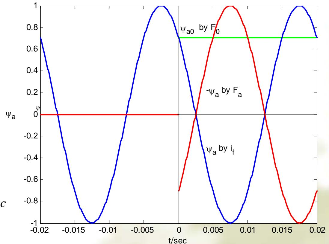
$$\psi_{a0} = \Delta\psi_a + \Psi_0 \cos(\omega t + \alpha_0) = [\psi_{a0} \text{ by } F_0]_{ap} + [\psi_a \text{ by } F_a]_\omega + \Psi_0 \cos(\omega t + \alpha_0)$$
