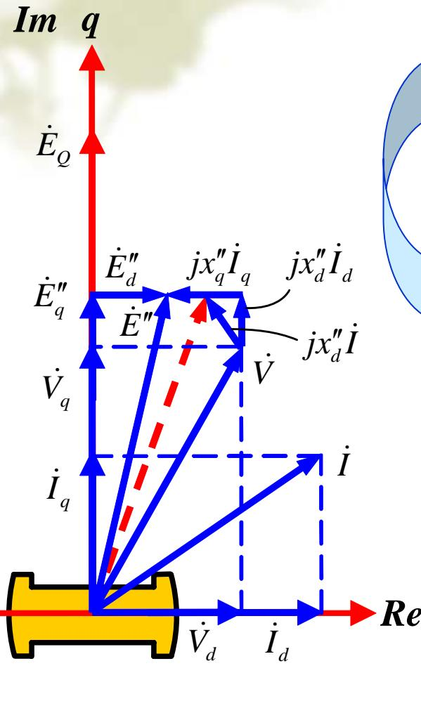
$$\begin{aligned} u_q &= E''_q - x_d'' i_d \\ u_d &= E''_d + x_q'' i_q \end{aligned}$$
