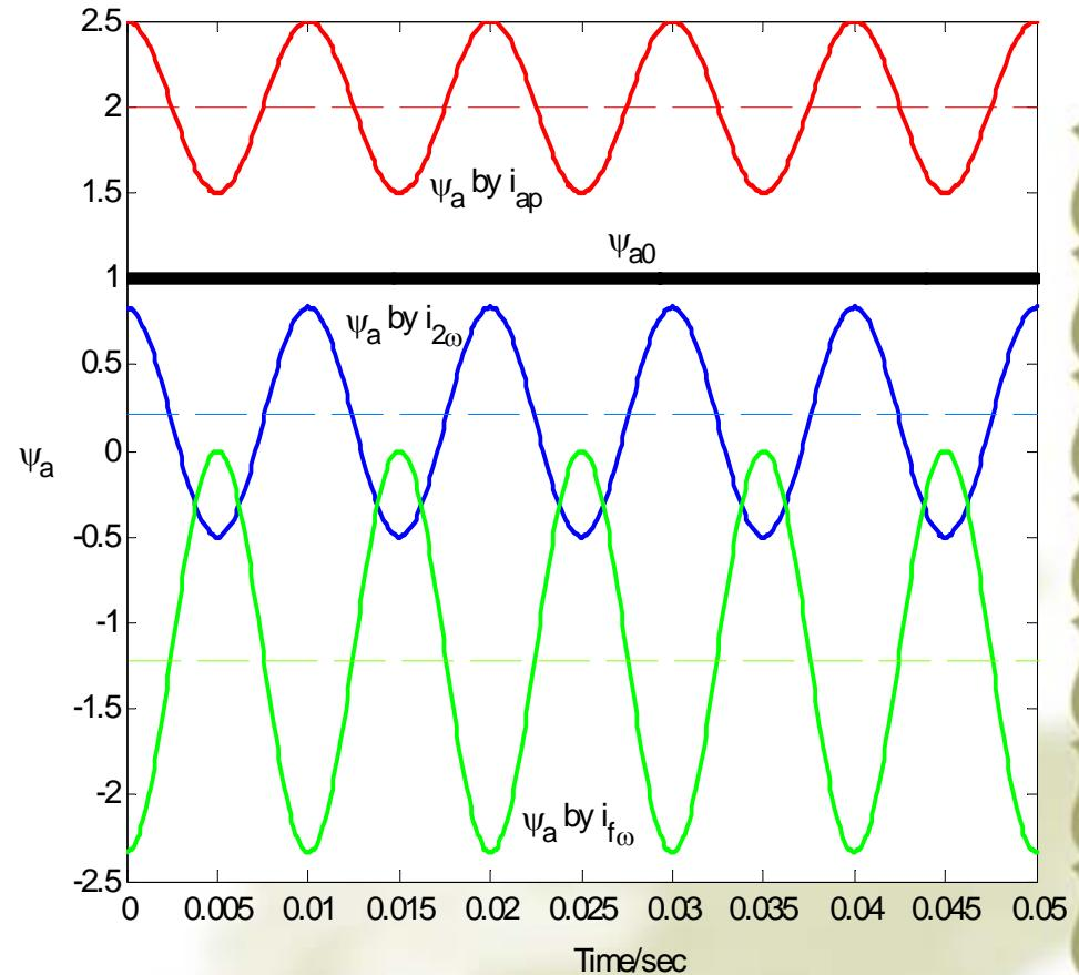
$$\psi_a = \psi_{(\omega)}^{i_{f[0]} + \Delta i_{fa}, i_{abc(\omega)}} + \psi_{(-)}^{i_{abc(ap)}, i_{abc(2\omega)}, \Delta i_{f\omega}} + \psi_{(2\omega)}^{i_{abc(ap)}, i_{abc(2\omega)}, \Delta i_{f\omega}} = \psi_{a0}$$
