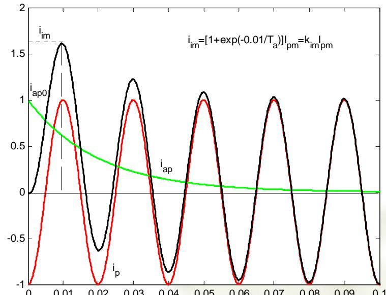
$$i = I_{pm} \sin(\omega t + \alpha - \varphi) + [I_m \sin(\alpha - \varphi') - I_{pm} \sin(\alpha - \varphi)] \exp(-t/T_a)$$
