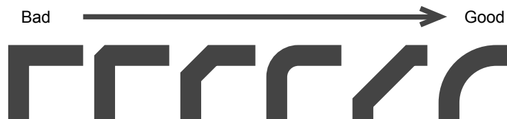
Figure 15. Layout of Corner wiring
