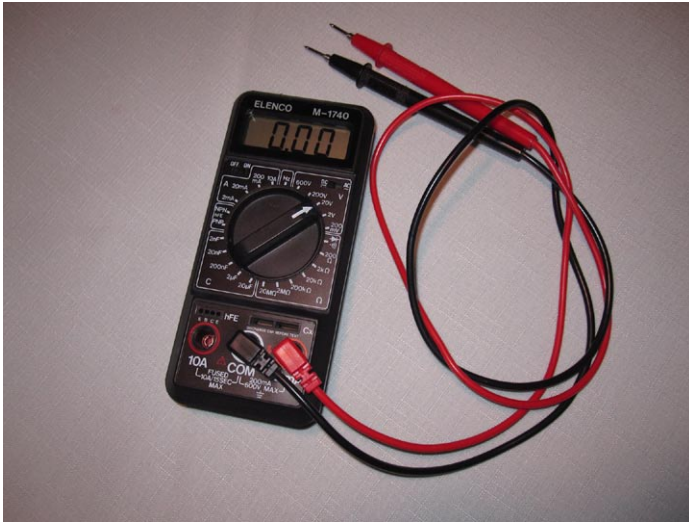
FIGURE 2.12 A low cost digital multimeter that measures DC and AC voltages, current, and resistance.
